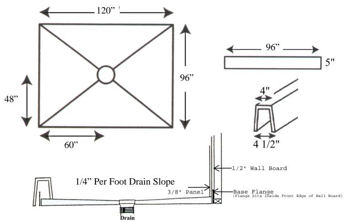
1 3/8" Outside Edge to 1/2" Thickness at Drain With no front threshold, this unit is ideal for handicap applications.
